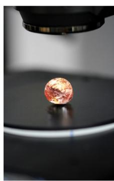
The testing of a colored gemstone Bellerophon at Gemlab involves a full range of analytical methods. Some are traditional, such as measuring the refractive index and specific gravity. Others involve state-ofthe-art techniques, such spectroscopy and laser-induced breakdown spectroscopy. Together, these combined techniques provide a deep understanding of the gemstone's properties.
